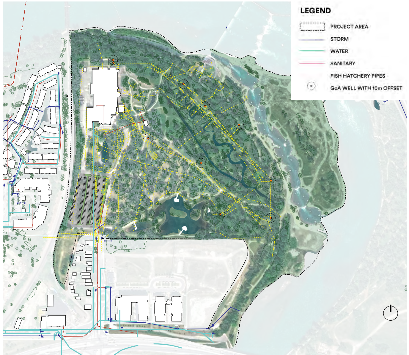
Figure 34: Site Plan Utilities - Deep
