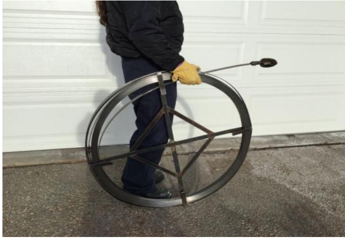
Figure 8: Water Services crew member displays the steel snake, a long coiled cable that is used to remove blockages.
