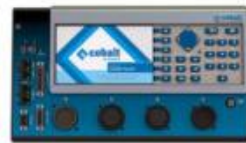
Figure 3: Intelight and Econolite Traffic Controllers (Sources: Q-Free America, Econolite Canada Inc.)
