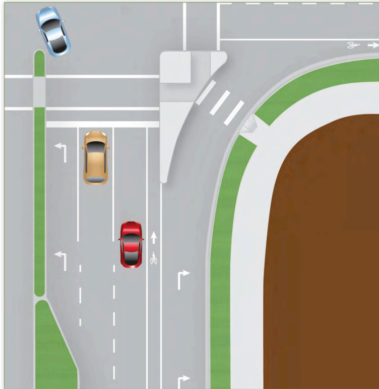
Traffic channelization is an effective mitigation strategy when intersection radii reduction is not an option. (Credit: Michele Weisbart)
