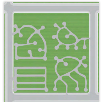
Cul-de-sac developments break up connectivity and create longer trips (Credit: Michele Weisbart)
