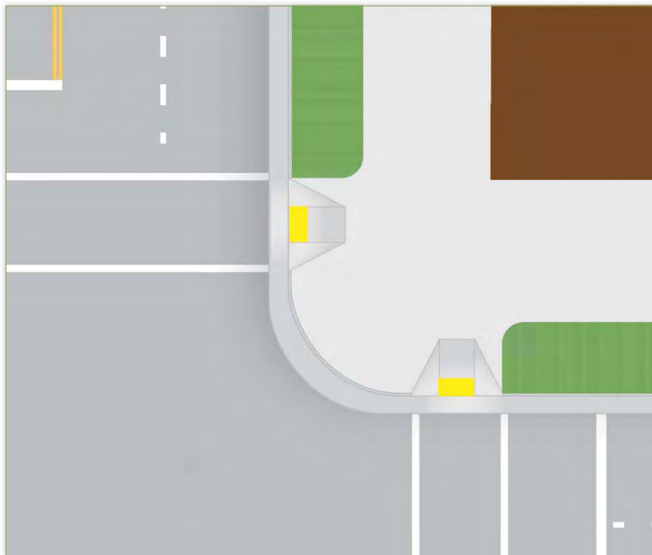
One curb ramp per crosswalk should be provided at corners. Ramps should align with sidewalks and crosswalks. (Credit: Michele Weisbart)
