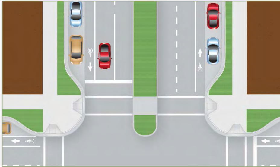
Integrating curb extensions and on-street parking into the sidewalk corridor enhances pedestrian safety and the walking experience. (Credit: Michele Weisbart)
