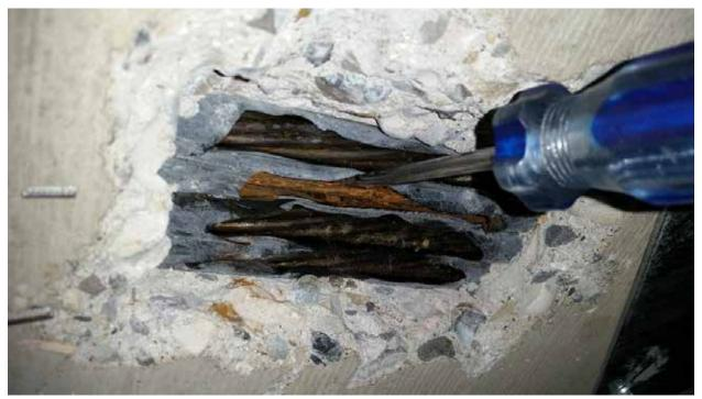
\*NOTE: Penetration test showing screwdriver wedged between wires of a post-tensioned strand. Note corrosion visible at the affected strand.
