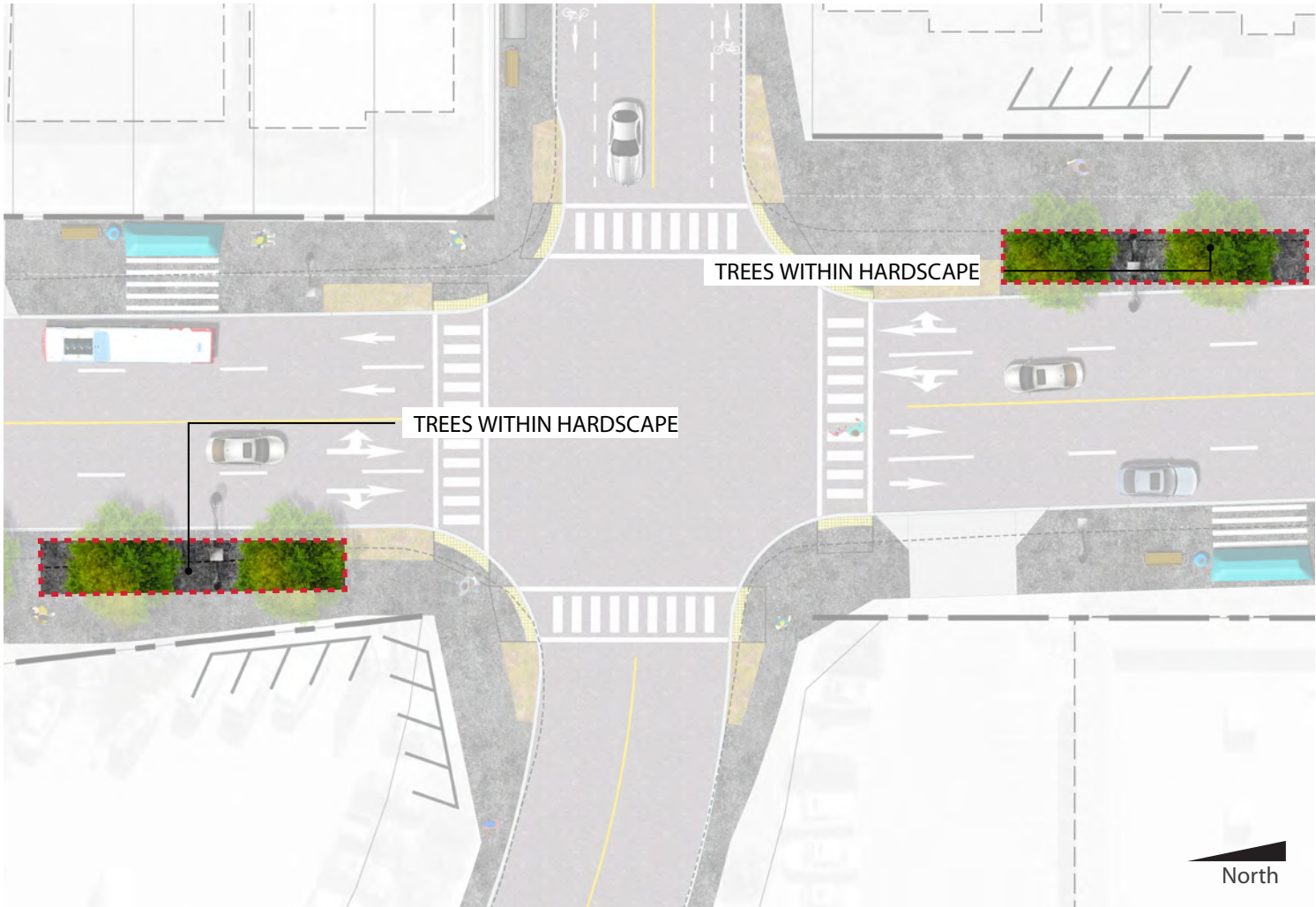
FIGURE 3.29 - TREE PLANTING SOIL CELLS CONCEPT PLAN
