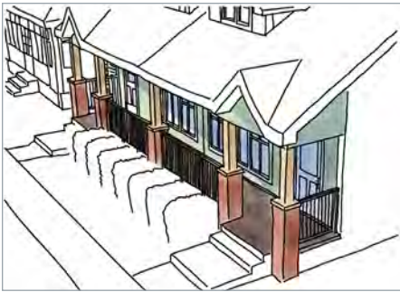
Full width verandah
