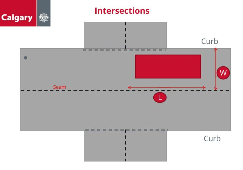
L = Minimum 10 m OR extend 1 m on both sides of the cut W = Curb to Closest Seam
