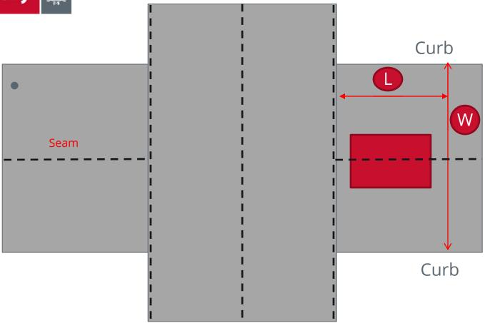
L = Minimum 10 m OR extend 1 m on both sides of the cut W = Curb to Curb
