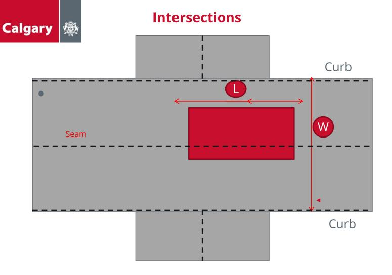
L = Minimum 10 m OR extend 1 m on both sides of the cut W = Curb to Curb
