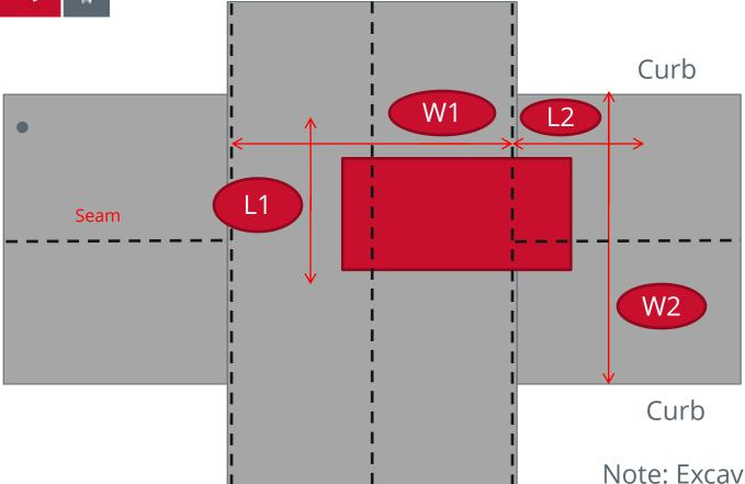
L = Minimum 10 m OR 1 m extension to both sides W = Seam to Seam OR Curb to Curb
