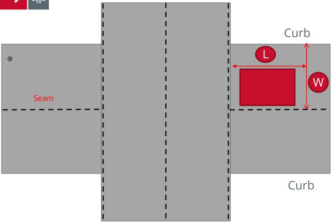
L = Minimum 10 m OR extend 1 m on both sides of the cut W = Curb to Closest Seam
