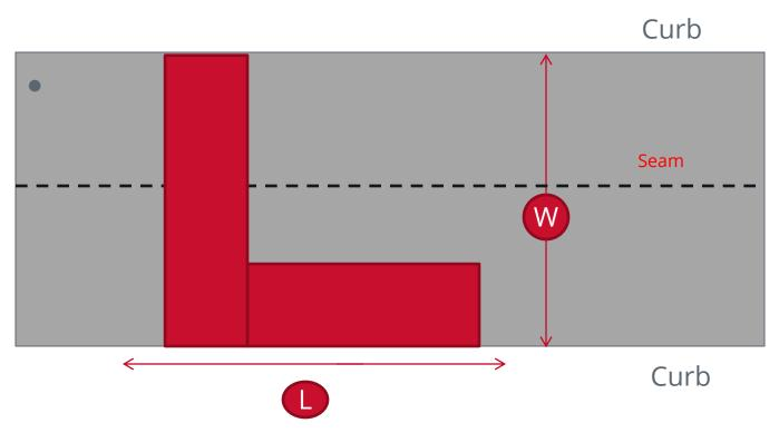
L = Minimum 10 m OR 1 m extension to both sides W = Curb to Curb
