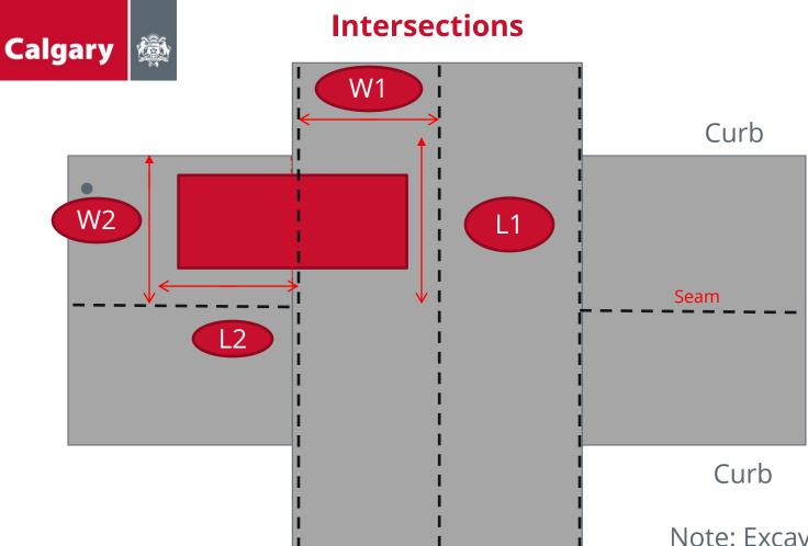
L = Minimum 10 m OR 1 m extension to both sides W = Curb to Closest Seam
