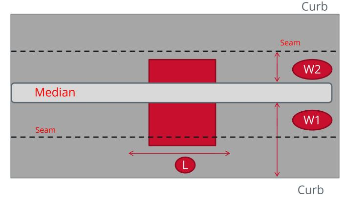
L = Minimum 10 m OR extend 1 m on both sides of the cut W = Curb to Closest Seam OR Curb to Curb
