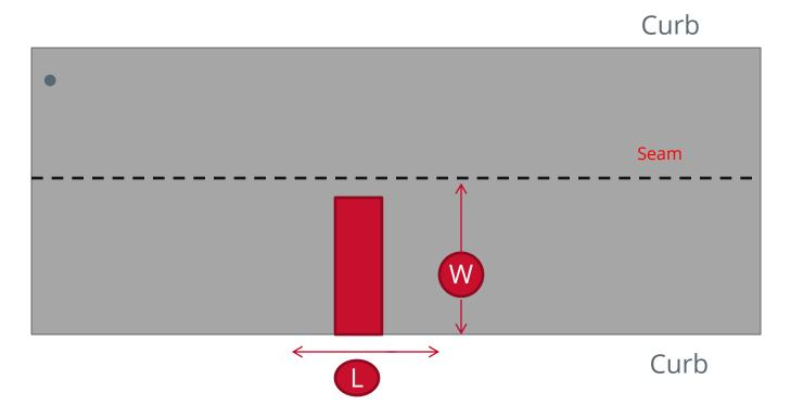
L = Minimum 10 m OR extend 1 m on both sides of the cut W = Curb to Closest Seam
