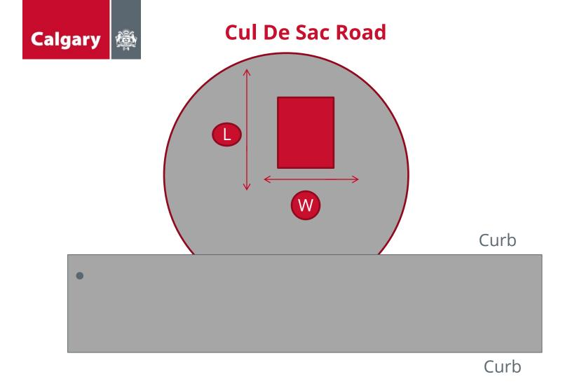
L = Minimum 10 m OR 1 m extension to both sides W = Minimum 3.7m or 1 m extension on both sides
