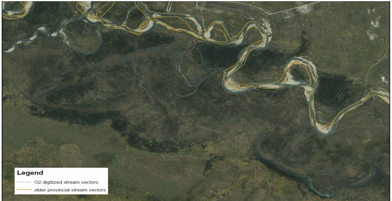
Figure 29. Sample Screenshot: Digitization of Stream Vectors to Improve Accuracy (light blue and orange lines)
