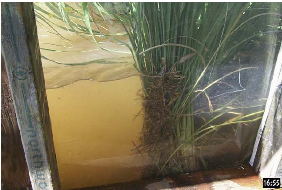
Figure 24. Visual of Suspended Solids Filtration by Vegetation (Source: State of Oregon)
